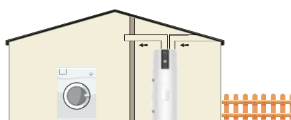
Installation with 2 ducts to the outside
